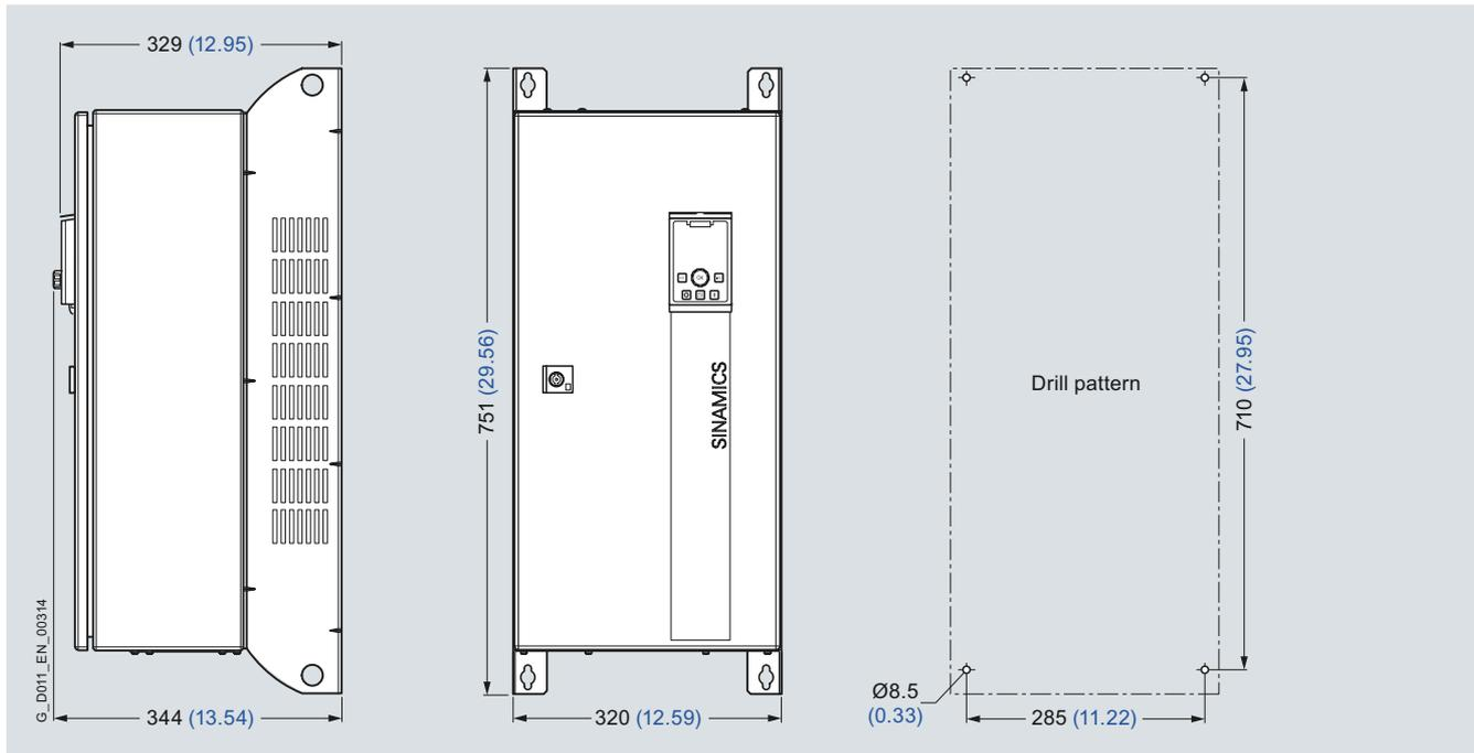
PM230 Power Module frame size FSE with integrated line filter class A/B
