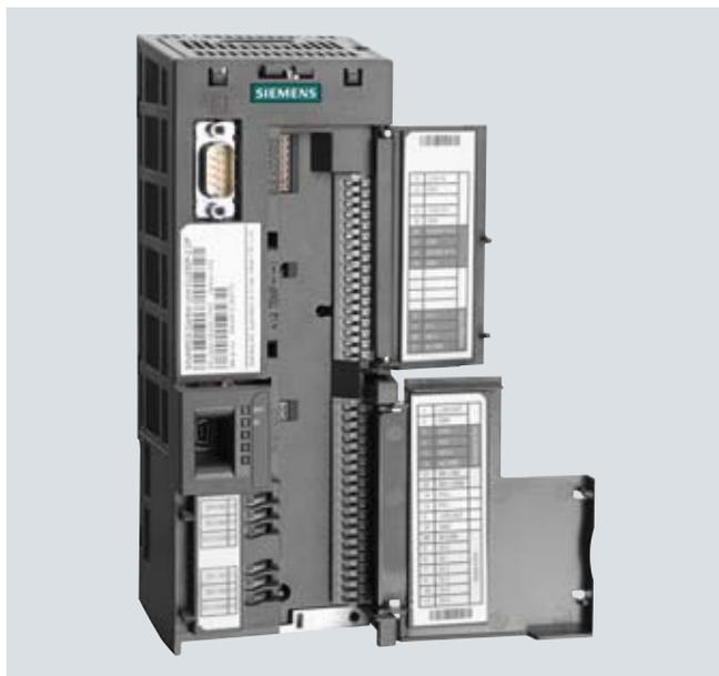
Example: CU230P-2 DP Control Unit with open terminal covers
