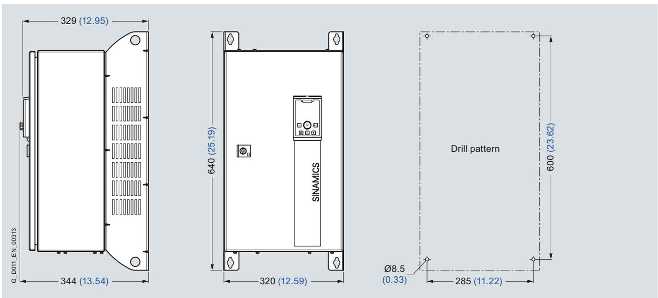
PM230 Power Module frame size FSD with integrated line filter class A/B
