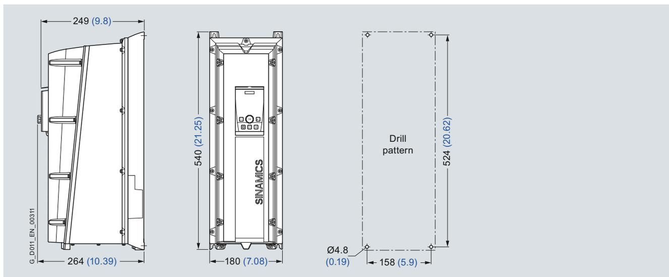
PM230 Power Module frame size FSB with integrated line filter class A/B
