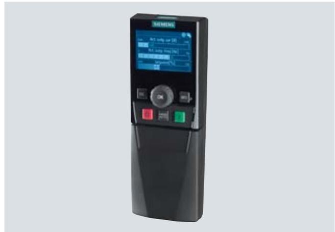
A handheld version of the IOP can be ordered for mobile use. In addition to the IOP, this includes a housing with rechargeable batteries, charging unit and RS232 connecting cable. The charging unit is supplied with connector adapters for Europe, the US and UK. When the batteries are fully charged, the operating time is up to 8 hours.
