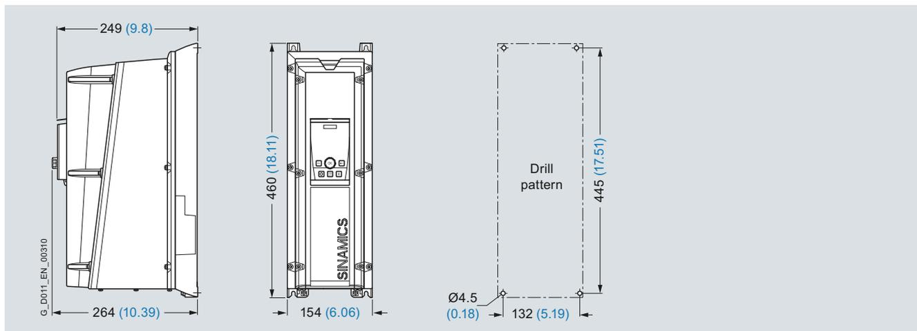
PM230 Power Module frame size FSA with integrated line filter class A/B
