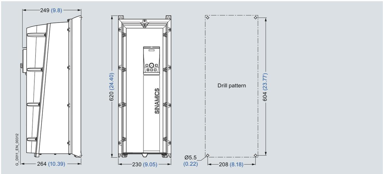
PM230 Power Module frame size FSC with integrated line filter class A/B
