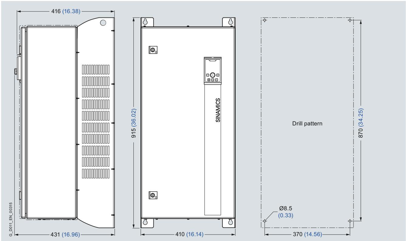
PM230 Power Module frame size FSF with integrated line filter class A/B
